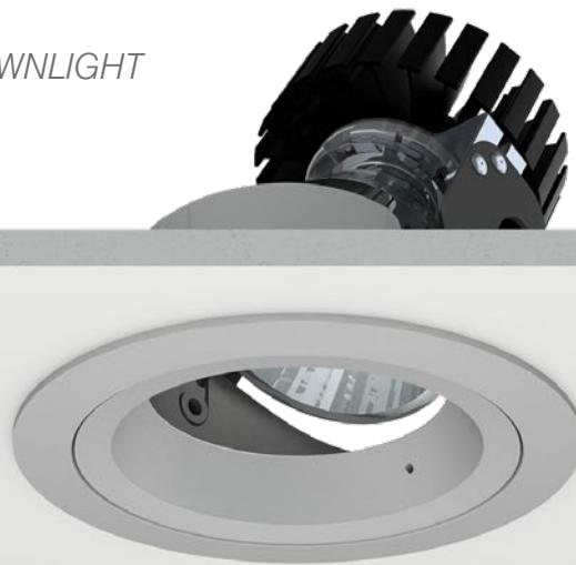
**Asteria 2 - Recessed Adjustable LED downlight.** The Asteria 2 gives you 360° of adjustment at a 40° angle. This new design allows you to choose your positioning and then lock the fixture in place. As a completely adjustable fixture, Asteria 2 is a great choice for unique designs where proper placement is critical.
