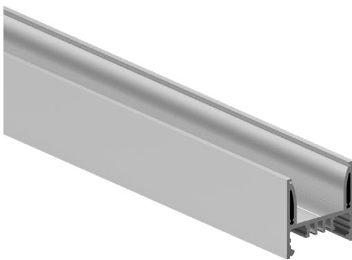
The KILO Channel is a linear aluminum extrusion that has been designed to fit many LED lighting needs and specifically high output applications. Substantial aluminum mass in profile provides excellent heat sink and physical protection for high power LEDs. The wide profile design can accommodate up to two rows of LED strips making the KILO extrusion ideal for bright general lighting applications. Extrusion and lens are field-cuttable. Channels come with specified Mounting Clips and End Caps.
