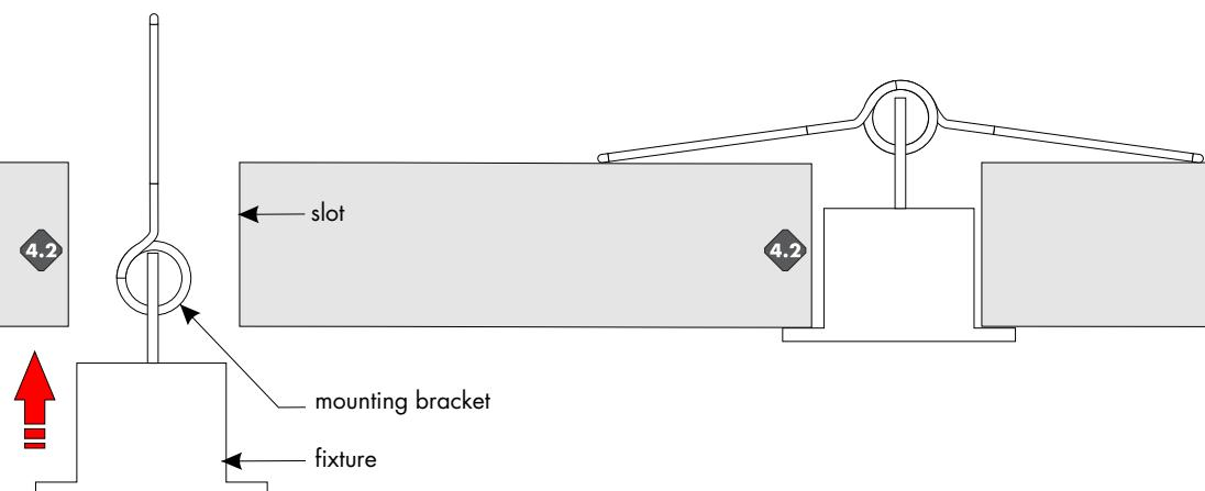
**4.3 For no surface mounting bracket option:** Apply construction adhesive to the bottom of the cutout slot, then place fixture onto adhesive to secure
