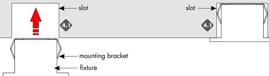
**4.2 For soft surface mounting bracket option:** Bend the adjustable springs to a straight position, followed by pushing the fixture completely inside the cutout slot. Then release the springs to secure.
