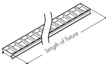
This White louver/lens combo comes in 12" increments and sits in place of a Myka lens, not in addition to.
