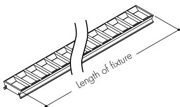
This Black louver/lens combo comes in 12" increments and sits in place of a Myka lens, not in addition to.
