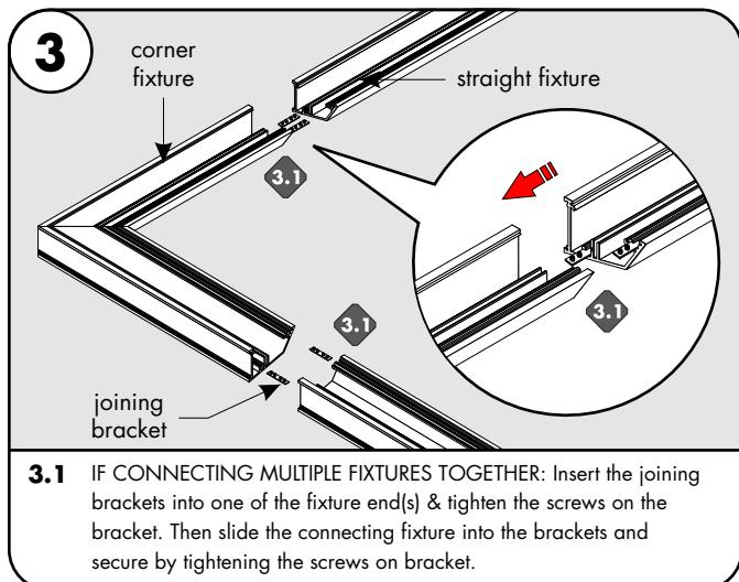
**3.1** IF CONNECTING MULTIPLE FIXTURES TOGETHER: Insert the joining brackets into one of the fixture end(s) & tighten the screws on the bracket. Then slide the connecting fixture into the brackets and secure by tightening the screws on bracket.
