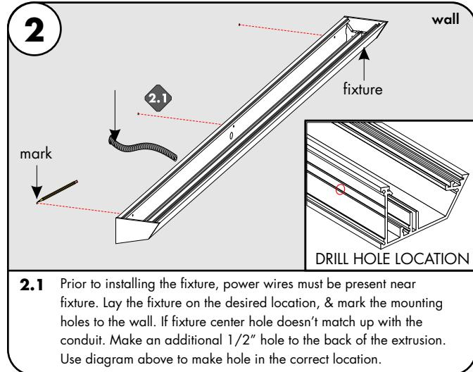
**2.1** Prior to installing the fixture, power wires must be present near fixture. Lay the fixture on the desired location, & mark the mounting holes to the wall. If fixture center hole doesn't match up with the conduit. Make an additional 1/2" hole to the back of the extrusion. Use diagram above to make hole in the correct location.
