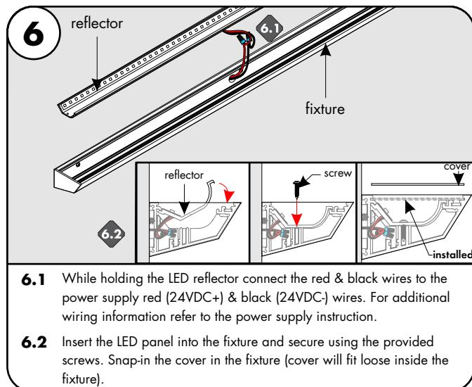
**6.1** While holding the LED reflector connect the red & black wires to the power supply red (24VDC+) & black (24VDC-) wires. For additional wiring information refer to the power supply instruction.
