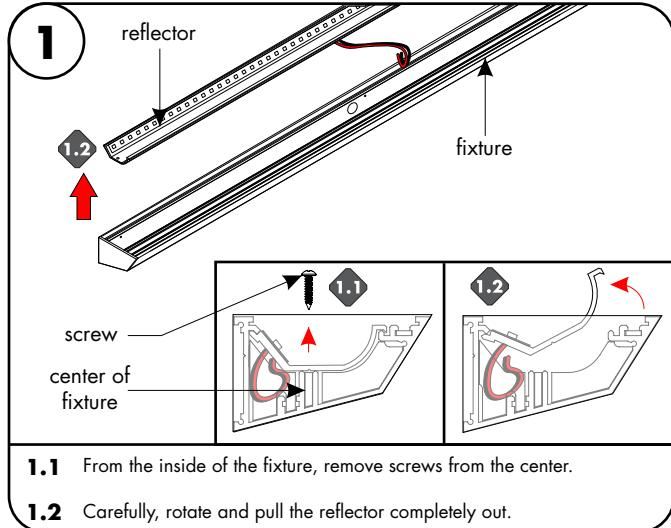
**1.1** From the inside of the fixture, remove screws from the center.
