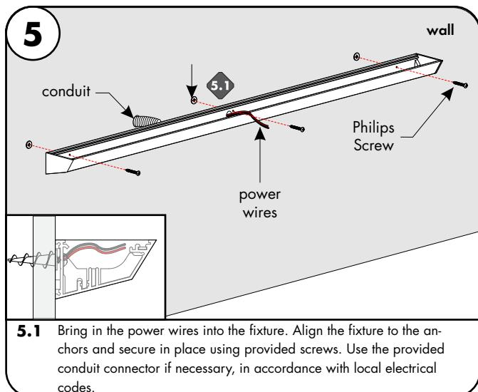
**5.1** Bring in the power wires into the fixture. Align the fixture to the anchors and secure in place using provided screws. Use the provided conduit connector if necessary, in accordance with local electrical codes.
