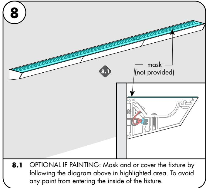
**8.1** OPTIONAL IF PAINTING: Mask and or cover the fixture by following the diagram above in highlighted area. To avoid any paint from entering the inside of the fixture.
