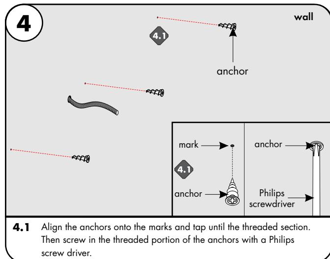
**4.1** Align the anchors onto the marks and tap until the threaded section. Then screw in the threaded portion of the anchors with a Philips screw driver.
