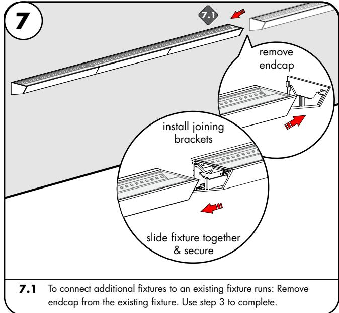
**7.1** To connect additional fixtures to an existing fixture runs: Remove endcap from the existing fixture. Use step 3 to complete.
