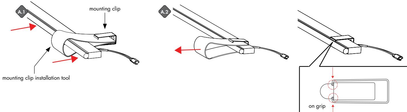
**A.1** Make an U shape with mounting clip installation tool, insert two edges into mounting clip. Place plexineon fixture inside the shape. Then push the fixture into clip.
