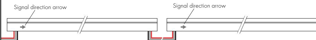
**NOTE:** Must power from the opposite direction of the signal direction arrow
