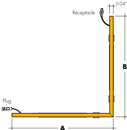
Note: Horizontal Corner legs are asymmetric, receptacle connector is on the longer end, plug connector is on the shorter end.
